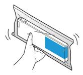
4. Push all the ink cartridges of the four colors gently into the product until they click in place. Check the color of the ink cartridge label and of the ink cartridge holder label, and set the cartridges to each matching color.
