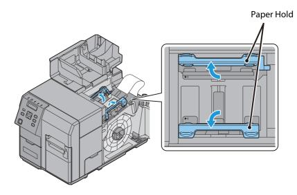
9. Insert the paper along the paper guide (a).Align the end of the paper with ▶| mark.
