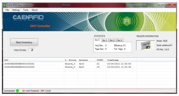
Fig. 2.2: CAEN RFID Easy Controller Side Bar
