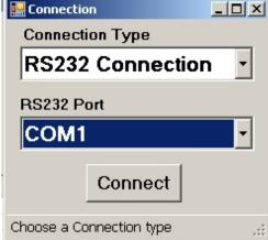
In the case of the serial port connection, the textbox above it is replaced by a combobox that lists all active serial ports.
