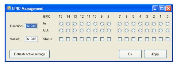
This window allows you to configure up to 16 GPIO (the number of enabled GPIO depends on the reader model). Direction and value are represented respectively by radiobutton and checkbox (if supported by the reader).
