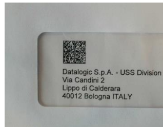
Figure 19 - Address Coded in Data Matrix Symbology for Automated Mail Processing
