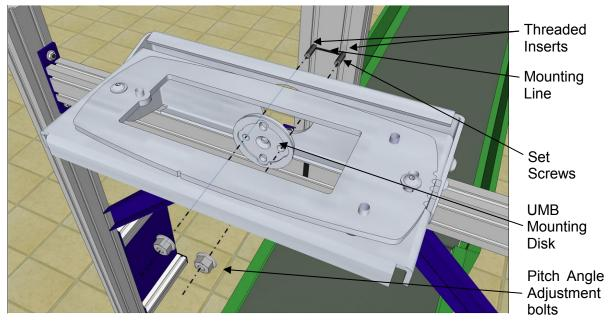
Figure 31: Securing the UMB to the structure
