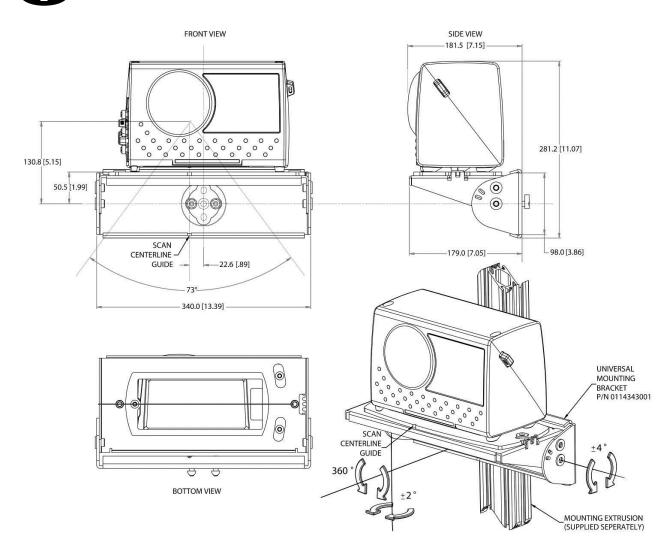
Figure 19: DM3610 Mounting Dimensions with UMB
