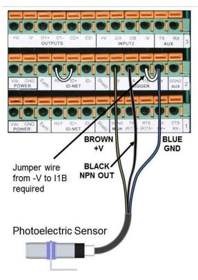
Figure 54: Photoelectric Sensor Wiring (PNP Output)
