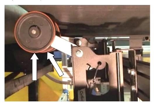
Figure 84: Tachometer Wheel
