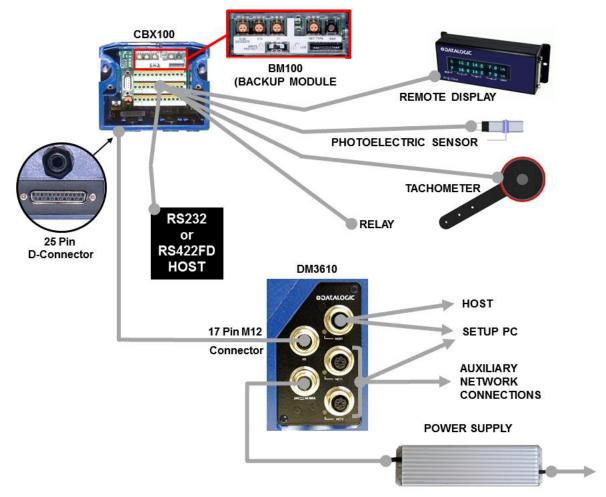
Figure 50: Wiring Block Diagram
