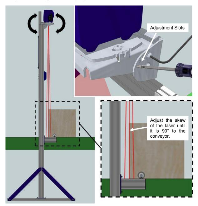
Figure 47: Adjusting the Skew
