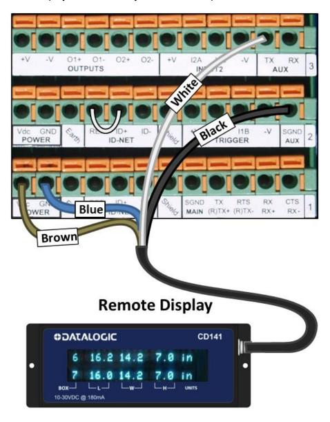
Figure 57: Remote Display Wiring
