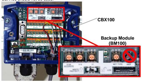
Figure 78: CBX100 with BM100 backup module installed
