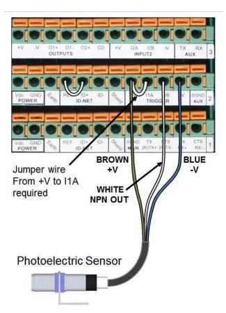
Figure 53: Photoelectric Sensor Wiring (NPN Output)
