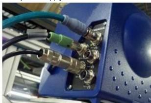
Figure 41: Connections to the DM3610 Connector Panel
