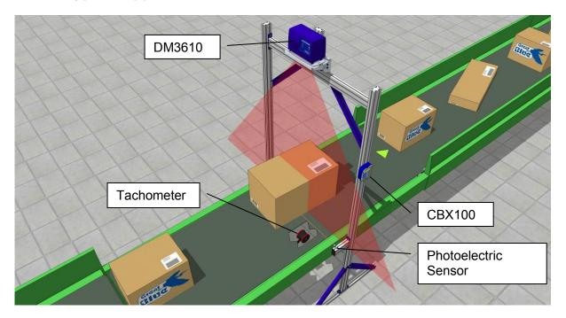
Figure 6: Typical DM3610 Installation (Singulated Version)
