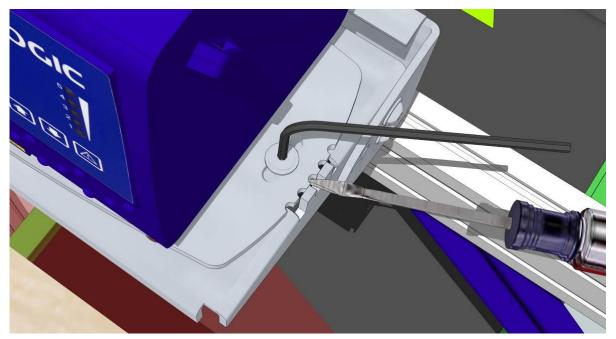
Figure 46: Adjusting UMB Mounting Plate with a Screwdriver
