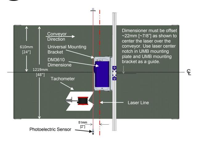
Figure 25: DM3610 Dimensioning System Installation - TOP VIEW
