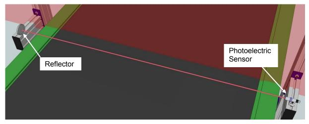
Figure 37: Mounting the Photoelectric Sensor
