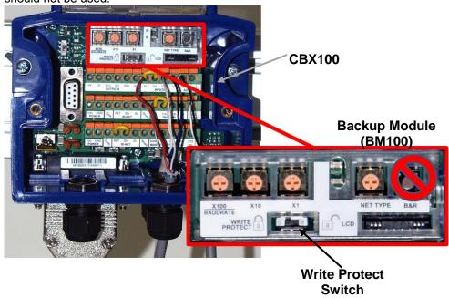
Figure 69: CBX100 with BM100 backup module installed
