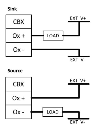
Figure 60: Isolated Relay Connection
