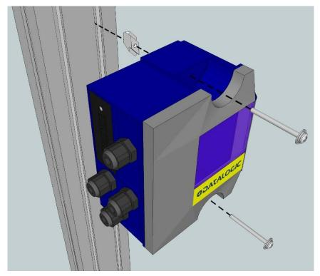
Figure 36: Securing the CBX100 using the 80/20 Mounting Kit
