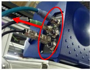
Figure 72: Remove Cables from DM3610
