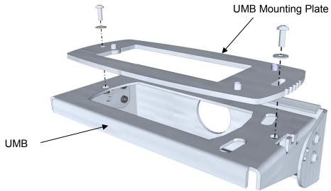
Figure 30: UMB Mounting Plate to UMB Assembly
