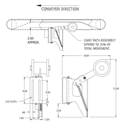
Figure 38: Tachometer Mounting Kit Installation
