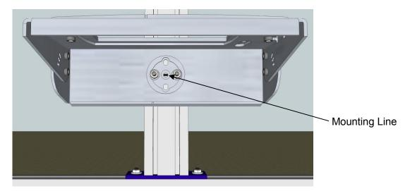
Figure 32: Aligning the UMB with the installation mark
