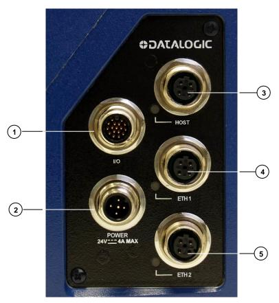
Figure 5: Connector Panel
