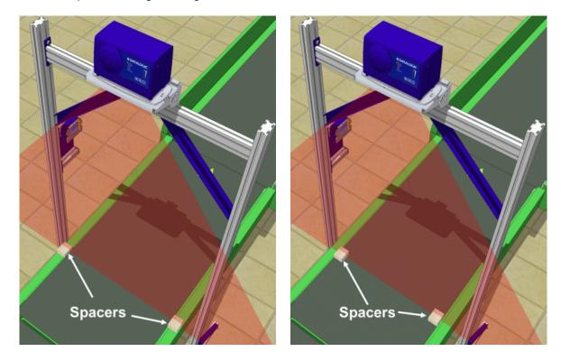
Figure 81: Placing the Spacers
