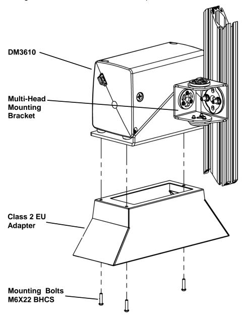
Figure 23: Class 2 EU Adapter Assembly with the Multi-Head Mounting Bracket
