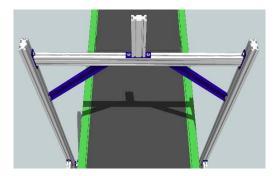
Figure 28: Center the Upright Mounting Support
