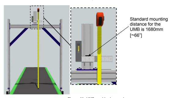
Figure 29: UMB positioning mark
