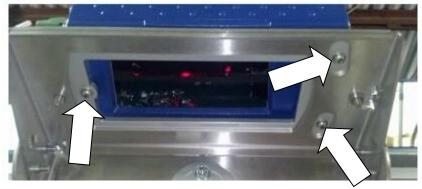
Figure 5.9: Mounting bolt location
