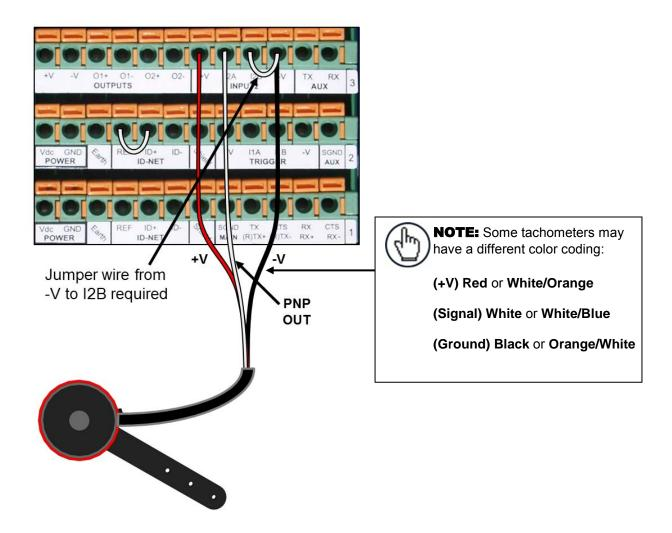
Figure 56: Tachometer Wiring (PNP Output)
