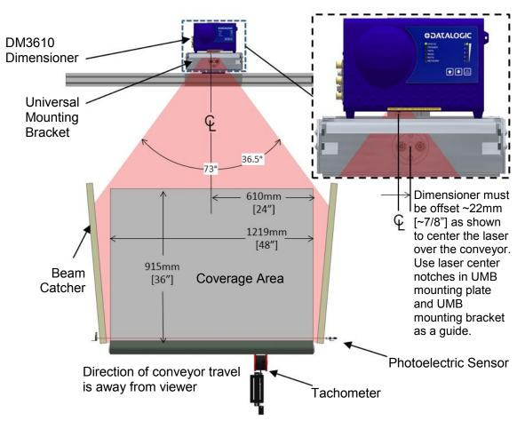
Figure 26: DM3610 Dimensioning System Installation - FRONT VIEW
