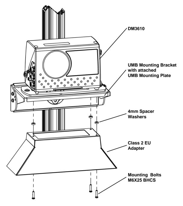
Figure 22: Class 2 EU Adapter Assembly with Standard UMB
