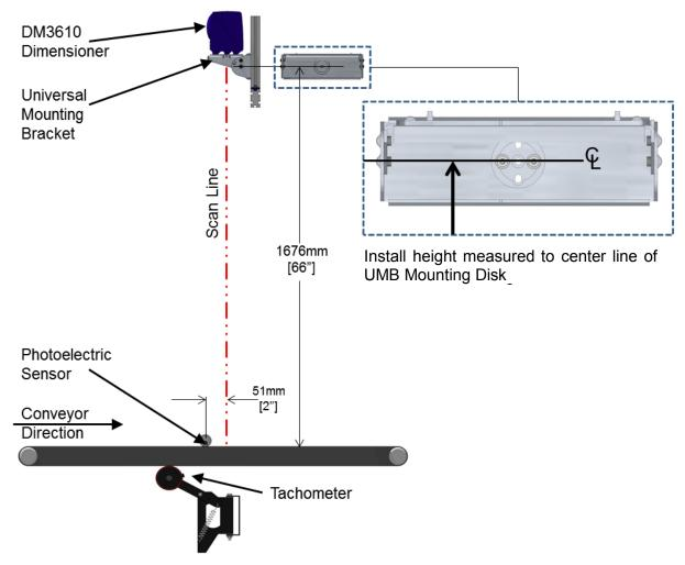
Figure 24: DM3610 Mounting Dimensions - SIDE VIEW
