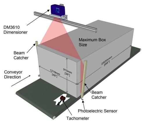
Figure 27: DM3610 Dimensioning System Installation - 3 QUARTER VIEW
