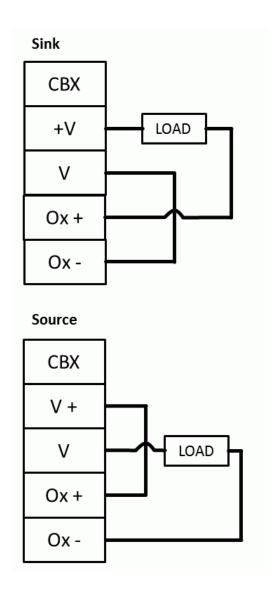
Figure 61: Non-Isolated Relay Connection
