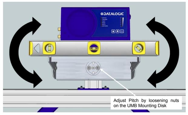
Figure 44: Adjusting the Pitch
