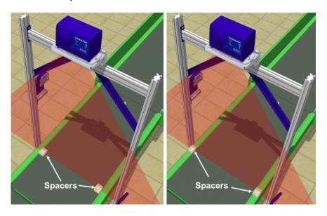
Figure 63: Side Margin Spacer Placement
