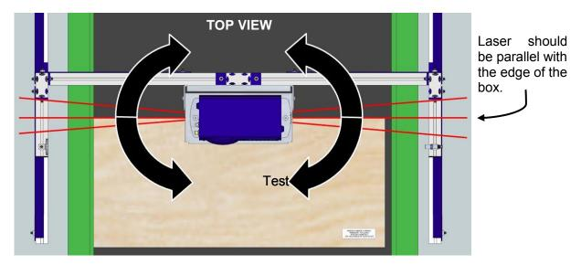
Figure 45: Adjusting the Tilt
