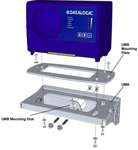
Figure 20: DM3610 and UMB Assembly
