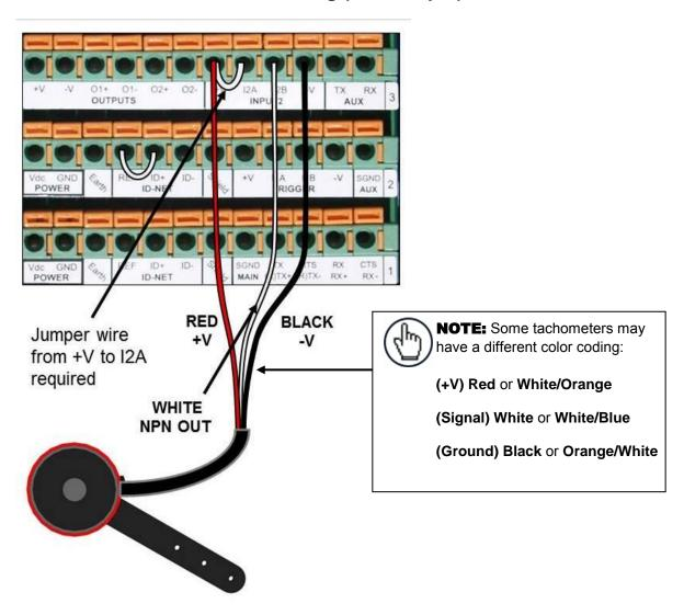
Figure 55: Tachometer Wiring (NPN Output)
