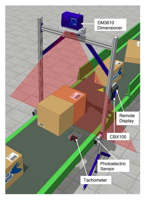
Figure 65: DM3610 Determining Package Height
