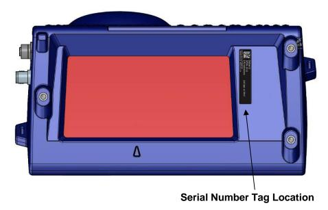
Figure 85: Serial Tag Location
