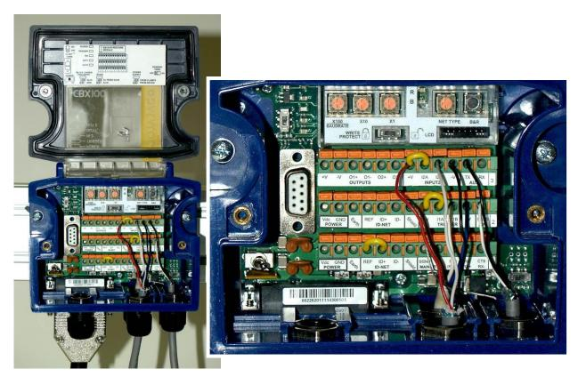
Figure 52: Securing wires with water-tight seals
