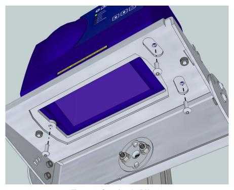
Figure 34: Securing the DM3610
