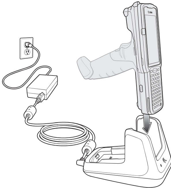
Figure 11 MC33XX Battery Charging
