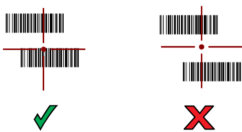
Figure 29 RS5100 Pick List Mode with Multiple Barcodes in Aiming Pattern
