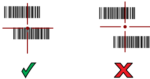
Figure 27 RS507/RS507X Pick List Mode with Multiple Barcodes in Aiming Pattern
