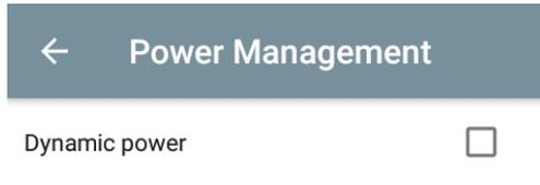
Dynamic Power optimization configures the reader for best battery life and works with Pre configured settings. Dynamic Power optimization works only for inventory operation
