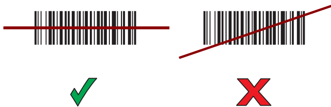
Figure 40 Laser Scanner Aiming Pattern
