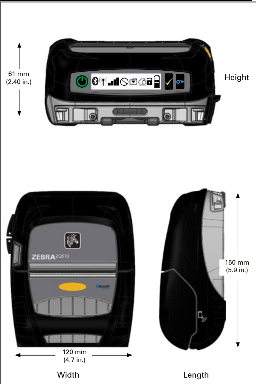
Figure 22: ZQ510 Overall Dimensions
