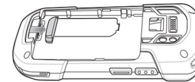
2. Insert the hand strap plate into the handstrap slot.
