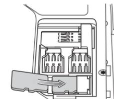
3. Replace the access door. Ensure that it is properly seated.
