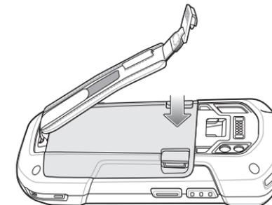
5. Place the hand strap clip into the hand strap attachment slot and pull down to lock in place.
