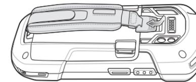
6. Lift the hand strap ribbon off the hook material.
