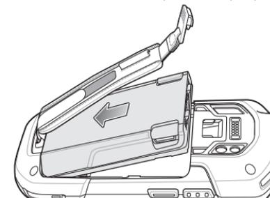
4. Rotate the battery down into the battery compartment and press the battery down until it snaps into position.
