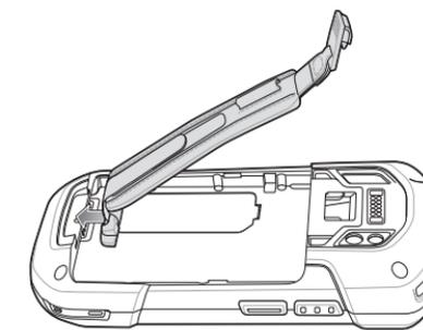
3. Insert the bottom of the battery into the battery compartment.
