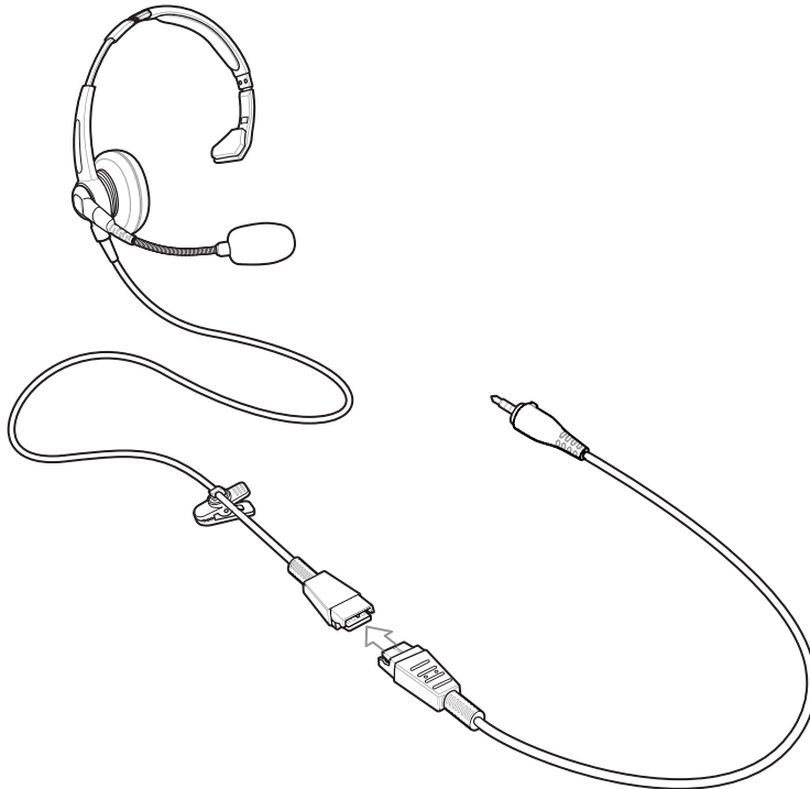
Figure 125: Connect Headset to Adapter Cable
