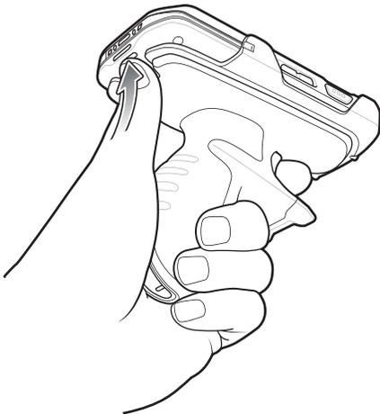
2. Slide the device away from the front of the Trigger Handle.
