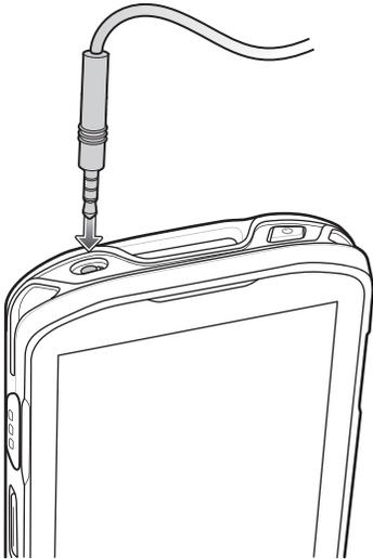
2. Connect the 3.5 mm connector plug of the headset into the 3.5 mm Audio Adapter.
