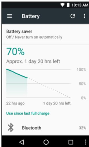
The **Battery** screen lists the applications using the battery. The discharge graph at the top of the screen shows the rate of the battery discharge since last charged (short periods of time when connected to a charger are shown as thin green lines at the bottom of the chart), and how long it has been running on battery power.
