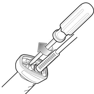
**Figure 1-8** Tightening Lock Plate into Unlocked Position
