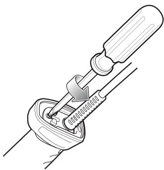
**Figure 1-6** *Loosening Lock Plate*
