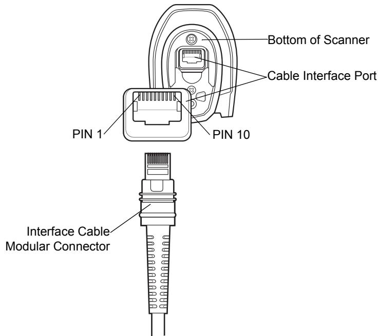
**Figure 3-1** Digital Scanner Cable Pin-outs
