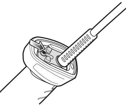
**Figure 1-4** Sliding Lock Plate into Locked Position
