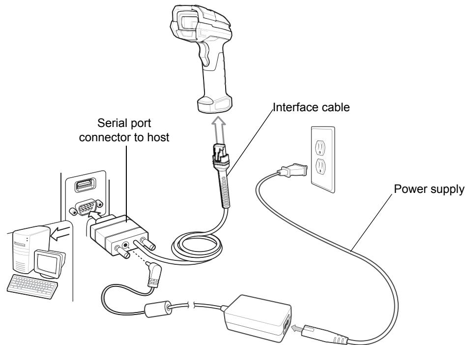
**Figure 8-1 RS-232 Direct Connection**
