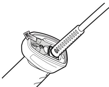
**Figure 1-7** *Sliding Lock Plate into Unlocked Position*
