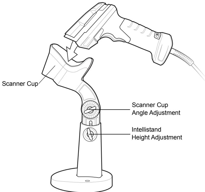
2. Insert the digital scanner in the Intellistand by placing the front of the digital scanner into the scanner cup (see [Figure 1](#)).
