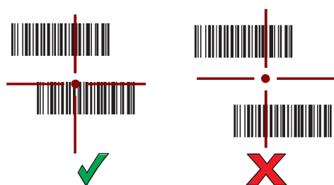
Figure 22 RS507/RS507X Pick List Mode with Multiple Barcodes in Aiming Pattern
