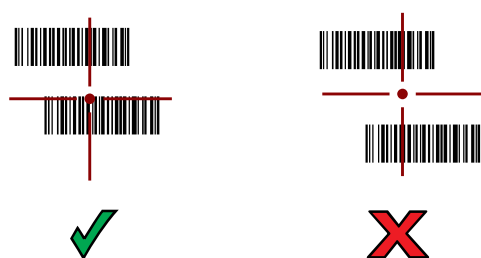
Figure 28 RS6000 Pick List Mode with Multiple Barcodes in Aiming Pattern
