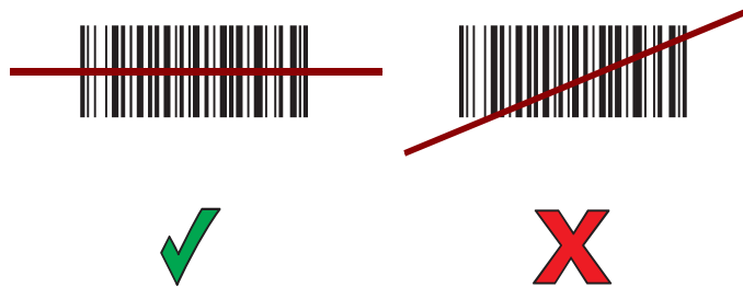
Figure 81 Linear Scanner Aiming Pattern
