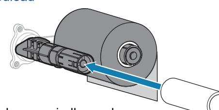
Place an empty core on the ribbon take-up spindle as shown. Push the core back as far as it will go.
