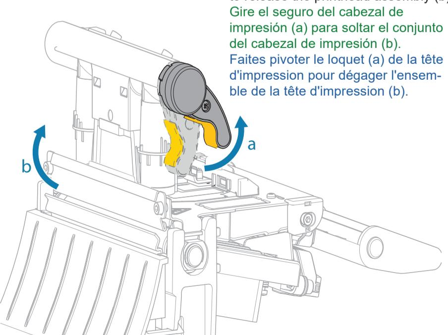
Rotate the printhead latch (a) to release the printhead assembly (b).
