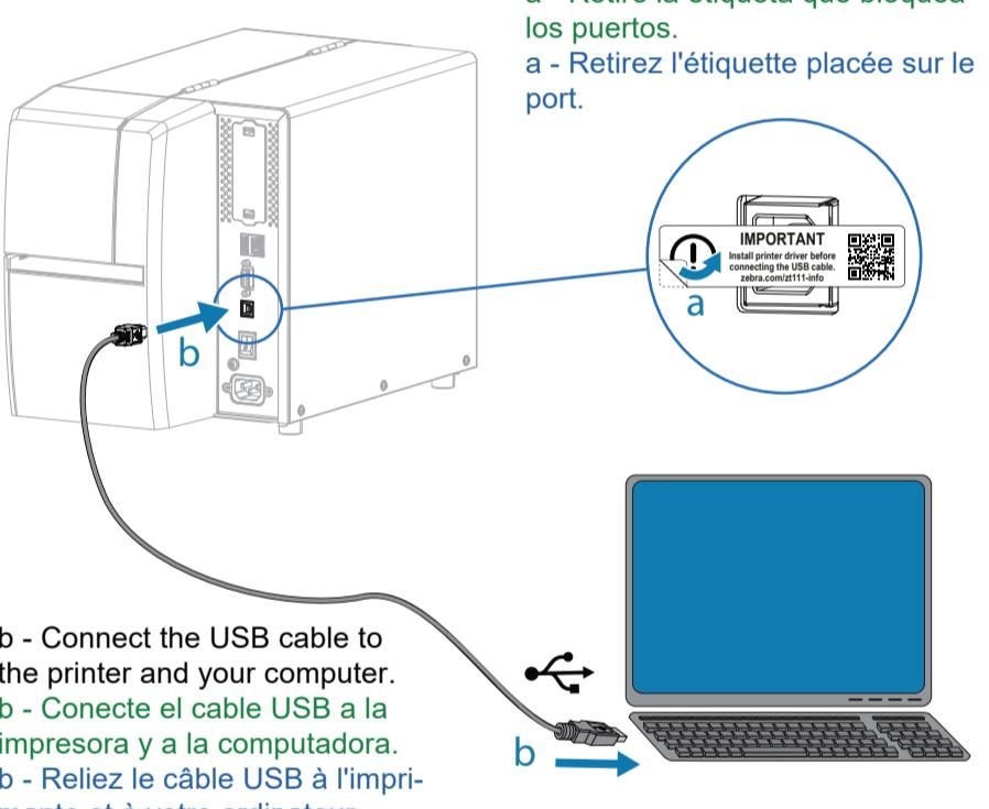
b - Connect the USB cable to the printer and your computer.
