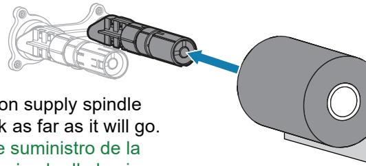
Place the ribbon on the ribbon supply spindle as shown. Push the roll back as far as it will go.
