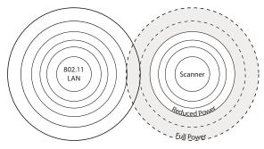
Scan one of the bar codes below to set the scanner's power output to **Full Power** (100%), **Medium Power** (35%), **Medium Low Power** (5%), or **Low Power** (1%). *Default = Full Power*.
