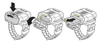
Replace the battery in the compartment, aligning the yellow dots on the battery and compartment, then slide the lock closed.
