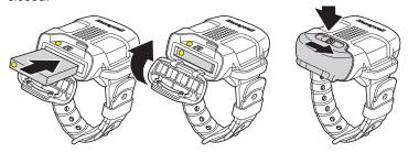
The 3.7V, 750mAh lithium ion battery in the Bluetooth module is designed to power the Bluetooth module for 8 hours and remain in standby for approximately 24 hours. Batteries are not fully charged when shipped. The battery should be charged for a minimum of 4 hours before initial use to ensure optimal performance.
