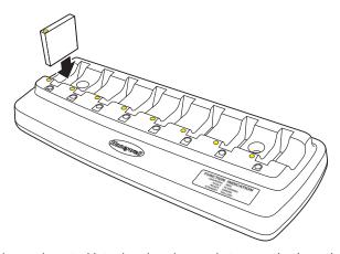
It is important that battery packs are inserted into the charging pocket correctly. Inserting the battery incorrectly could result in damage to the battery pack or the charger.
