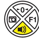
**Step 3.** Press the **F1** button. The LCD display shows **CALIBRATE SCALE – SINGLE RANGE KGS**.
