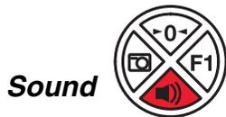
Press repeatedly to scroll through the beeper volumes. This button is also used to clear error conditions (LED lights, beeps, and LCD notifications). Hold this button down for 5 seconds to put the scanner to sleep.
