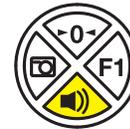
**Step 8.** The LCD display leads you through the next step of placing a full weight of 30 lbs. on the scale. The LEDs flash 3 times. Press the **Sound** button once the scale weight settles on full weight.
