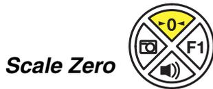
This button is normally lit when the scale is at zero. The backlight goes off when the scale is not at zero. Press this button to reset the scale to zero.
