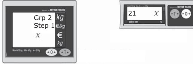
**Step 2.** Either display will initially display **x = NO**. Press the Tare **+T+** key to change this to **YES**:
