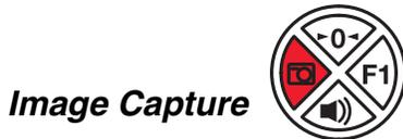
Press this button once to scan a bar code using a customer-facing scanner (if installed). Push it a second time to disable the customer-facing scanner. See [Image Capture Button](#) on page 4-7 for further information.
