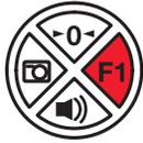
Press this button once quickly to input a number of repeat scans. For example, if there are 6 cans, the cashier would scan the first can, then push the F1 button 5 times quickly to indicate 5 more repeats of that scan. Press and hold the F1 button for 5 seconds to deactivate an EAS tag. Refer to [F1 Programmable Button](#) (page 4-4) for further information about the F1 button settings.
