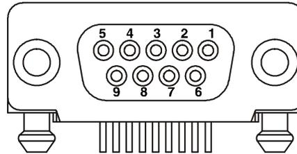
*Note: The signal names are referenced to the terminal. The terminal is a DCE RS232 device. Refer to section, RS232 Communications Cables and RS232 Pin Configuration for more details. The base is at a right-angle to the printed circuit board (PCB). The ninth pin has a ring indicator (RI).*
