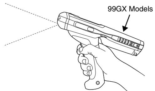
3. Project the aiming beam or pattern by pressing and holding one of the following:
