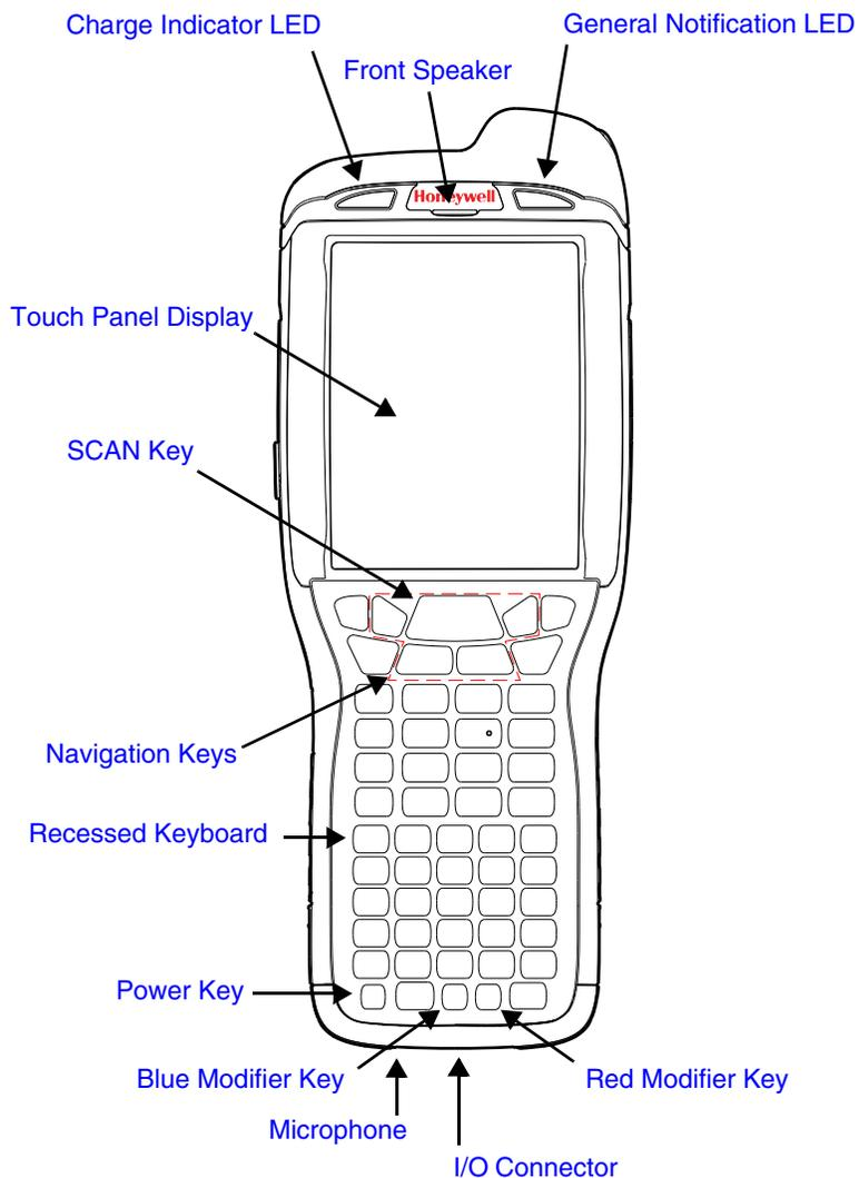
Note: The illustration above shows the 55-Key Full Alpha/Numeric Keyboard option. For a complete overview of the optional keyboards available for the 99EX/99GX, see [Using the Keyboards](#) on page 5-1.
