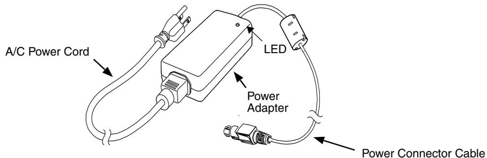
1. Plug the A/C power cord into the power adapter.
