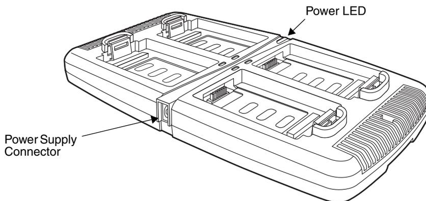
4. The power LED illuminates green, and the charger performs a self-diagnostic test that lasts approximately five seconds.
