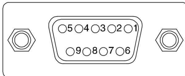
*Note: The signal names are referenced to the terminal. The terminal is a DCE RS232 device. Refer to section, RS232 Communications Cables and RS232 Pin Configuration for more details. The ninth pin has a ring indicator (RI).*
