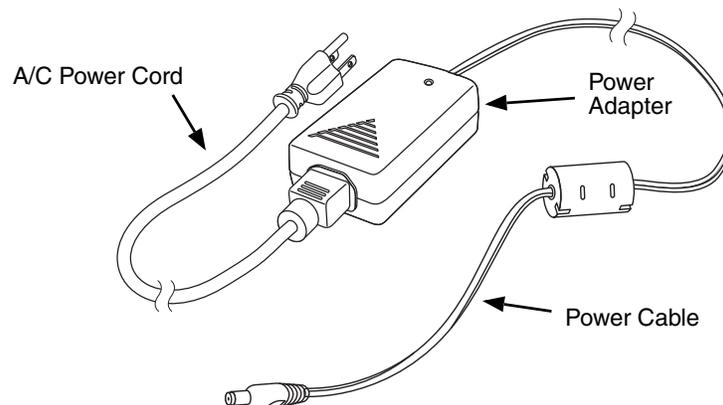
1. Plug the A/C power cord into the power adapter.
