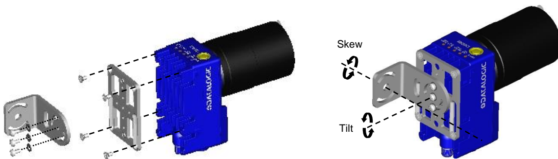
Figure 28 –Positioning with Matrix 450N Body Mounting Bracket (Back)
