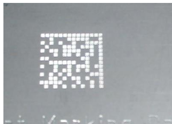
Figure 19 - Dot Peening Marking on Metal Surface with Multi-dot per Code Element
