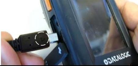
Connect the Single Slot Dock to the peripheral by means of a Micro-A USB cord, or use a Micro-A to Std-A receptacle USB adapter such as Datalogic 94A051969 (together with a standard USB cable if needed).
