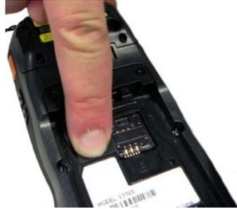
5. First insert the bottom (contacts) and then the upper side of the battery pack into the slot. Press until the battery latch clicks.
