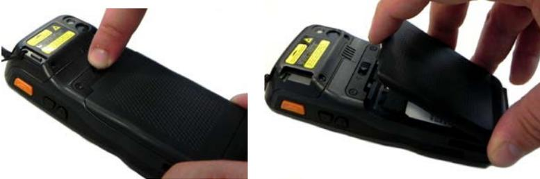
3. Open the card slot and insert the microSD card with the written part downward:
