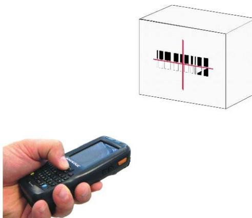
The Lynx Imager uses an intelligent aiming system pattern, similar to those on cameras, indicating the field of view, which should be positioned over the code:
