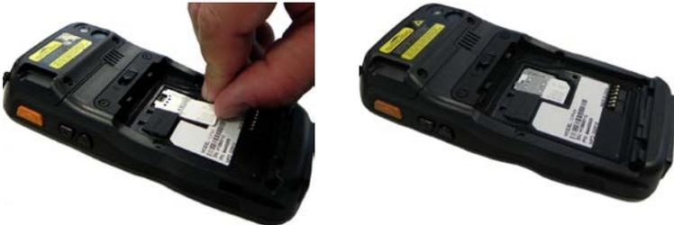
4. First insert the bottom (contacts) and then the upper side of the battery pack into the slot. Press until the battery latch clicks.
