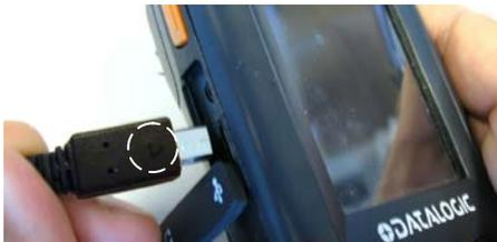
The Single Dock can be connected to the Host by means of the Micro-B USB cord 94A051968.
