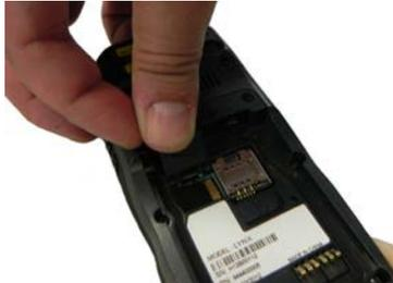
4. Shift the card to the right to lock it into the cardholder; close the card slot:
