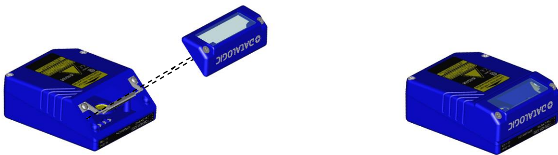
Figure 19 - Mounting a GFC-2020 Deflection Mirror
