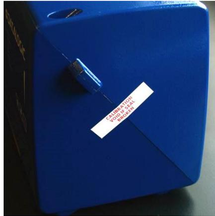
If required, adhesive-backed, paper tamper-proof seals may bridge the seam between the two halves of the housing, on opposite sides of the device.
