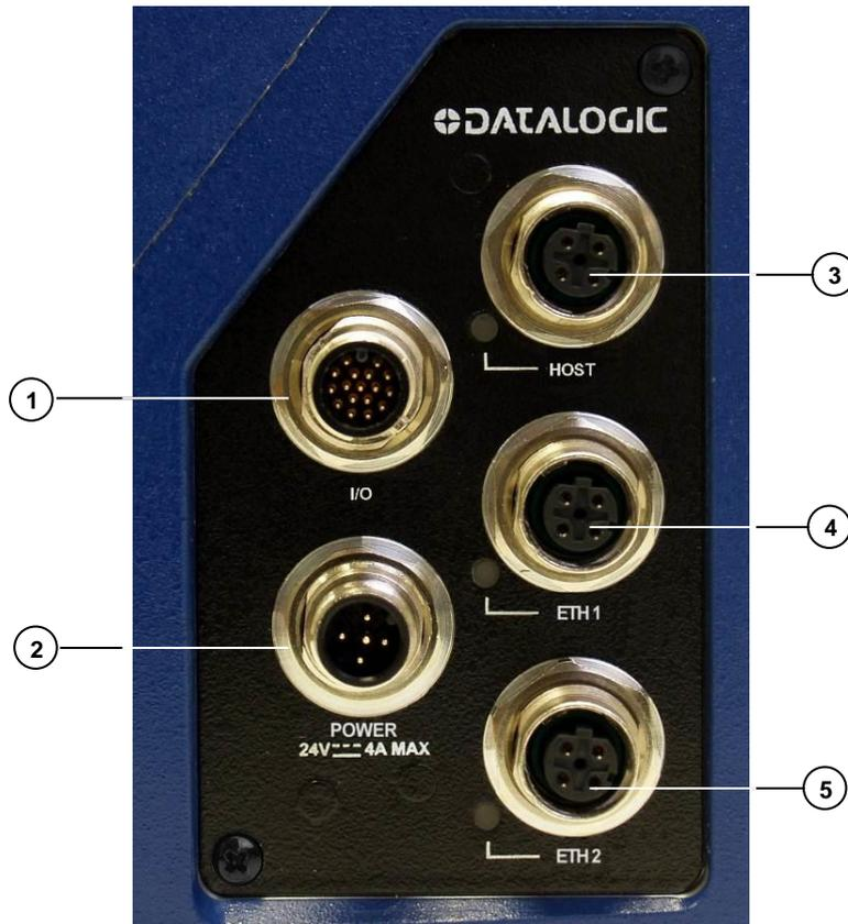
**Figure 5: Connector Panel**
