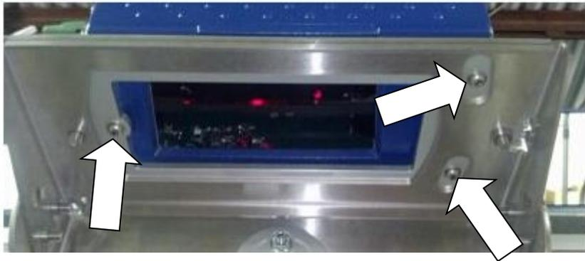
Figure 5.9: Mounting bolt location
