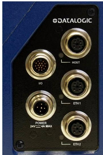
Figure 62: Connector Panel
