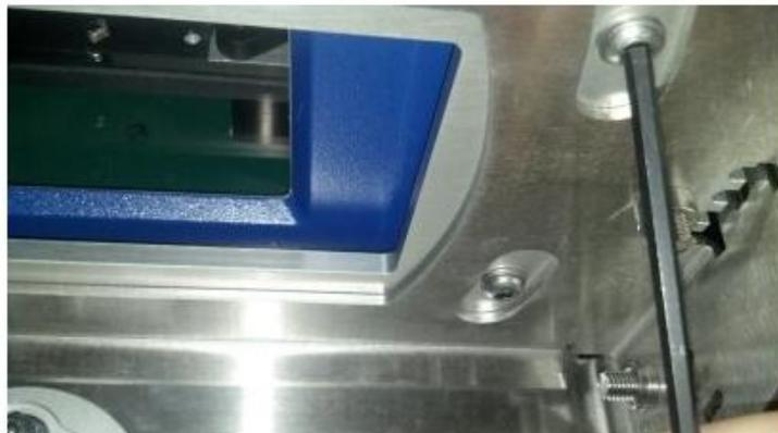
Figure 73: Removing a mounting bolt
