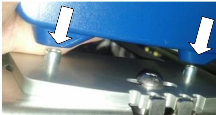
Figure 74: Placing DM3610 on the hollow Spirol™ spring dowel
