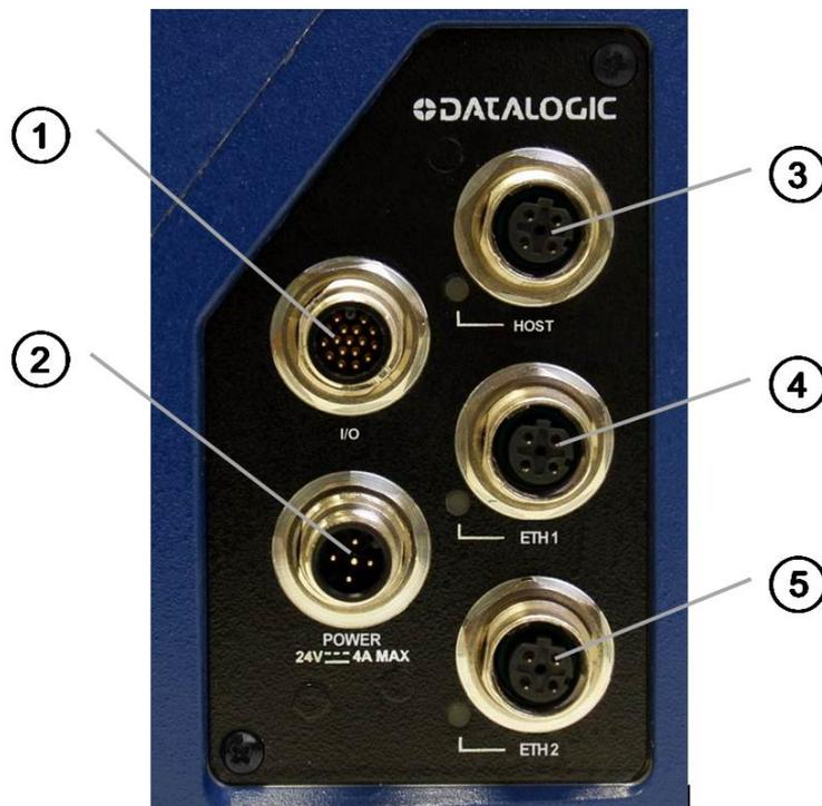
Figure 48: DM3610 Connector Panel
