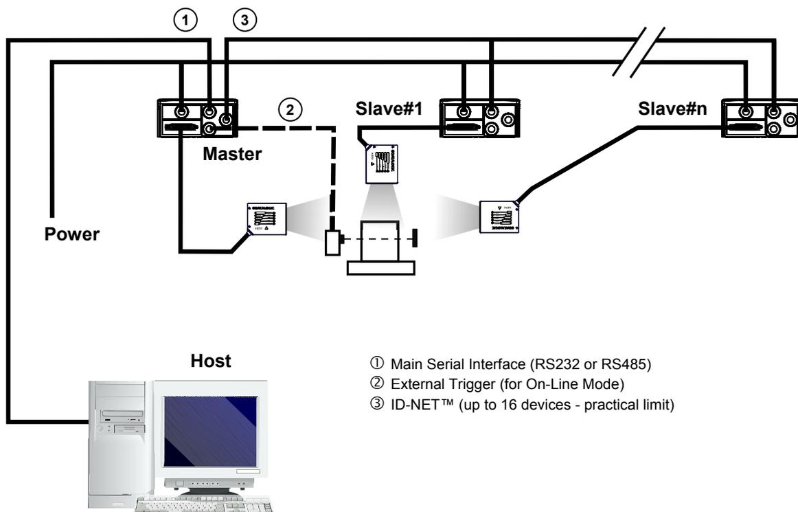
The ID-NET™ interface allows local connection of multiple scanners that are reading on different sides of the same target. All scanners share a single presence sensor and activate/deactivate simultaneously.
