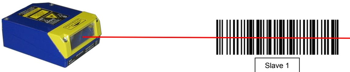
3. Once the scanner has successfully read the code, the LEDs stay on steady for 2 seconds:
