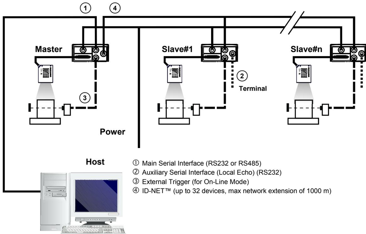
The ID-NET™ interface allows connection of scanners that are reading objects placed on independent conveyors. All scanners are typically located far away from each other and they use a dedicated presence sensor.
