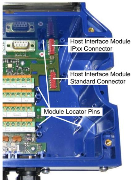
Figure 2 – CBX500 Host Interface Module Mounting References
