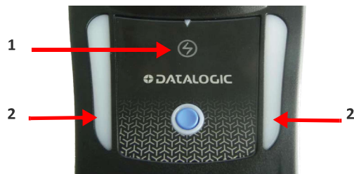
Figure 12 - Gryphon Base LEDs
