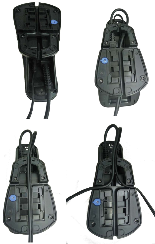
Figure 6 – Options for routing the DC cord
