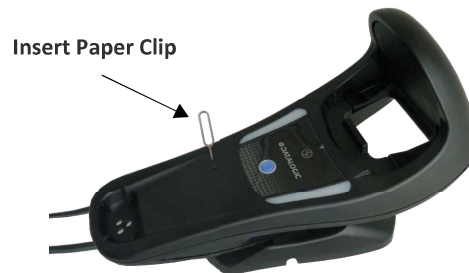
Figure 8 - Disconnecting the Cable
