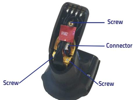
3. Carefully lift out the gold contacts circuit, and remove the battery holder while letting the white connector pass through the hole in the battery holder (as shown below).
