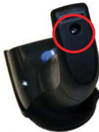
2. Unplug the three screws securing the battery holder, and unplug the white connector.
