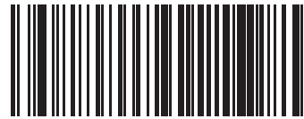
Codabar Quiet Zones = Quiet Zones on two sides
