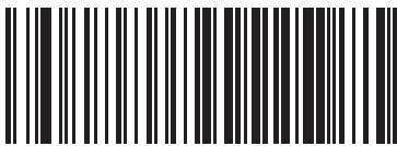
Codabar Quiet Zones = Small Quiet Zones on two sides
