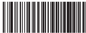
GS1 DataBar™ Expanded Minimum Reads = 3
