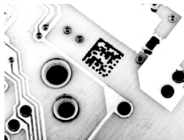
Figure 23 - Data Matrix Code Directly Marked on PCB Surface by Using Laser Etching Technology
