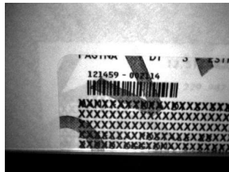
Figure 18 - Overprinted Barcode Readable by Matrix 210™ also Through the Envelope Window Film
