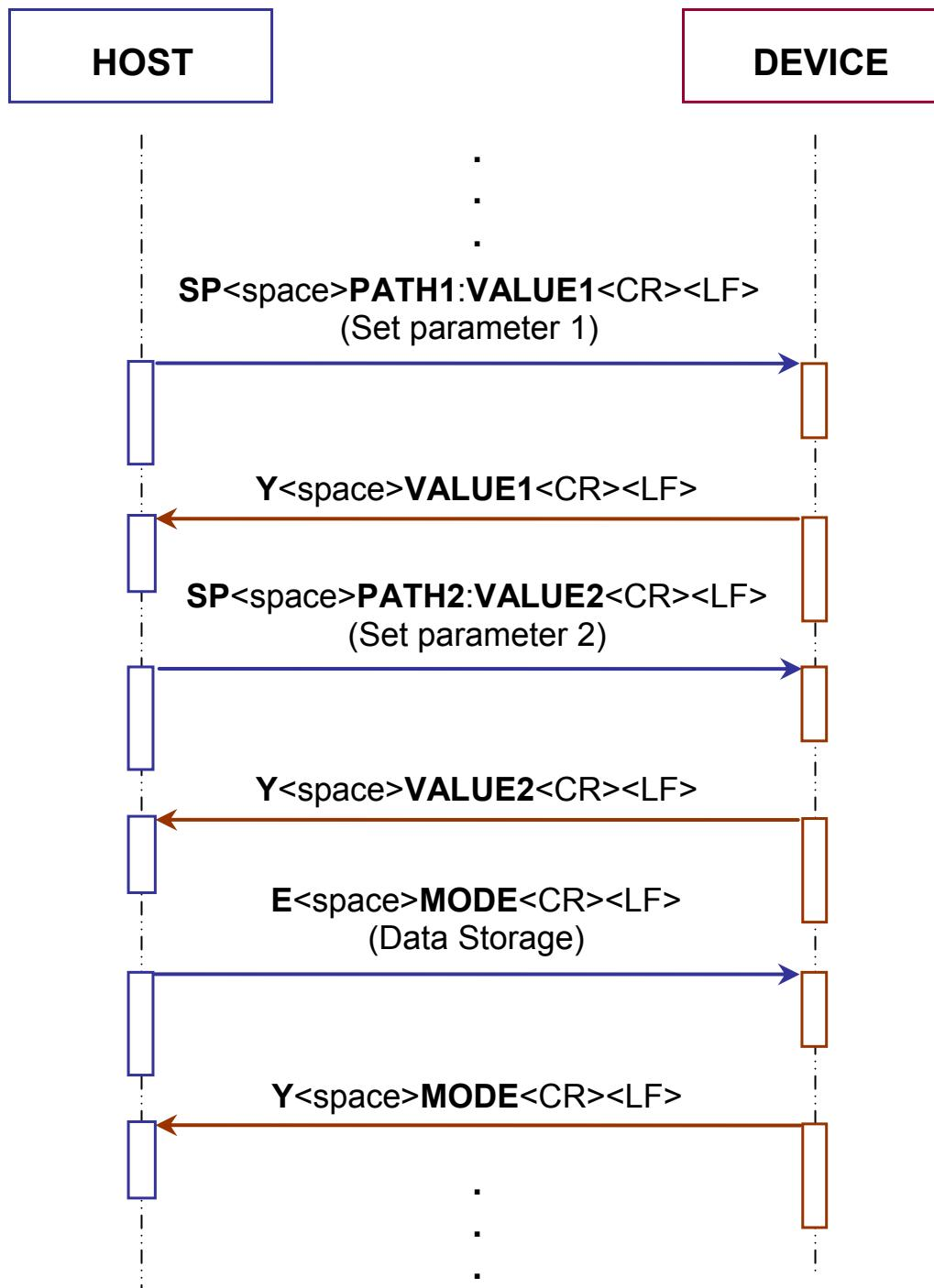
Figure 3 - Two Parameters Programming Session With Data Storage
