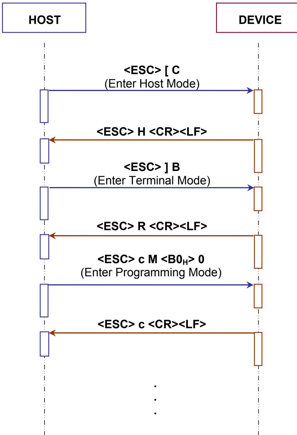
Figure 1 - Connection to Stand Alone Device
