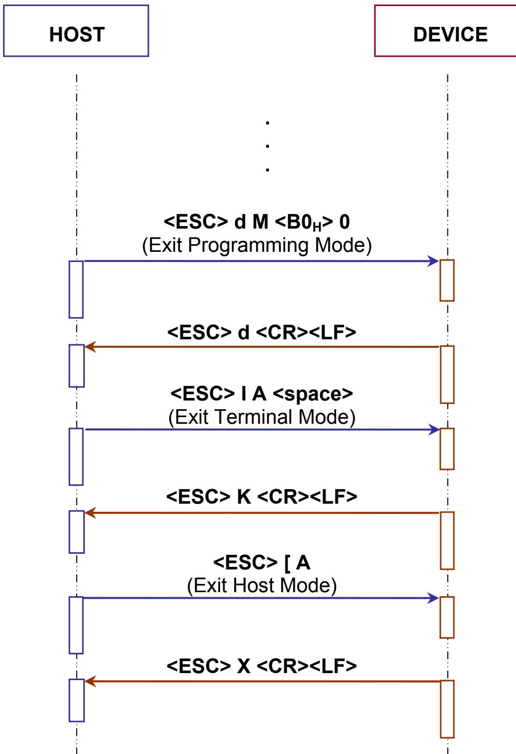
Figure 2 - Disconnection from Stand Alone Device
