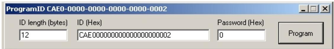
*Note:* EPC Class1 Gen2 defines two types of password: “kill password” and “access password” and both are 4 byte long. If a tag is locked, “access password” is used for all the operations but killing; kill operation must be performed using the “kill password”. The two passwords are stored in a reserved bank of tag.
