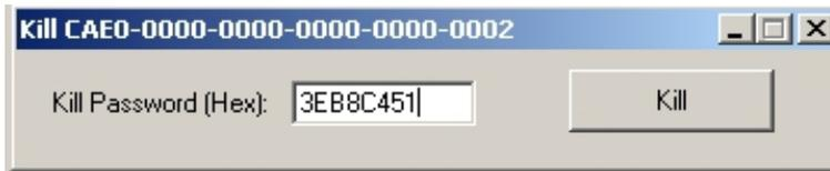
This window provides a password textbox and a *Kill* button; type the password (4 bytes in hexadecimal format i.e. A013B4F9) in the textbox and press *Kill*.
