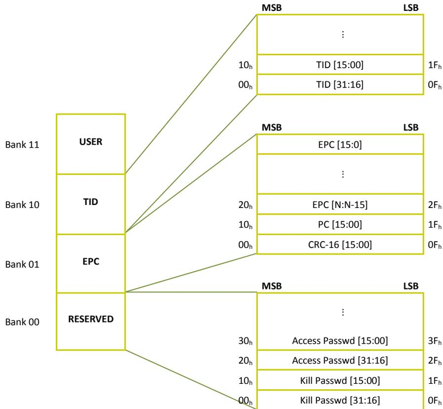
The inventory process returns the EPC code that is part of the content of the EPC memory bank as a side-effect of the singulation process. All the memory content, anyway, can be read using the Gen2 Read command and the rewritable memory can be written using the Gen2 Write command.
